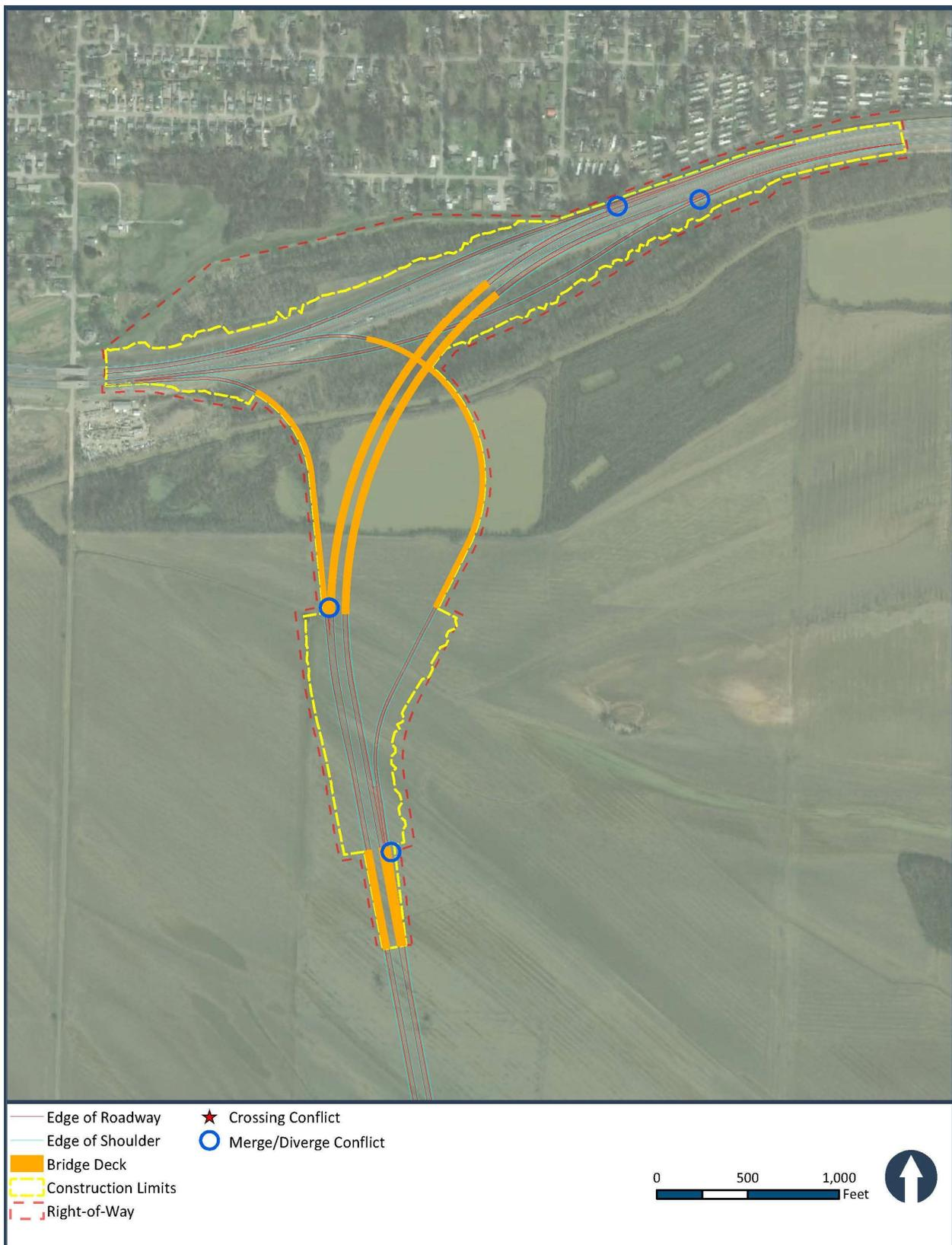
**Figure 2-2. VMP Concept B: Modified System Interchange with Right-Hand Exit**
