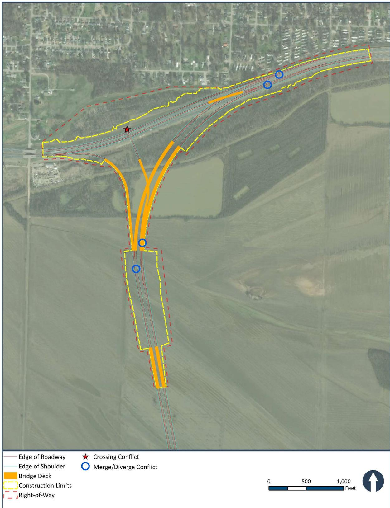
**Figure 2-5. VMP Concept E: Service Interchange 2**
