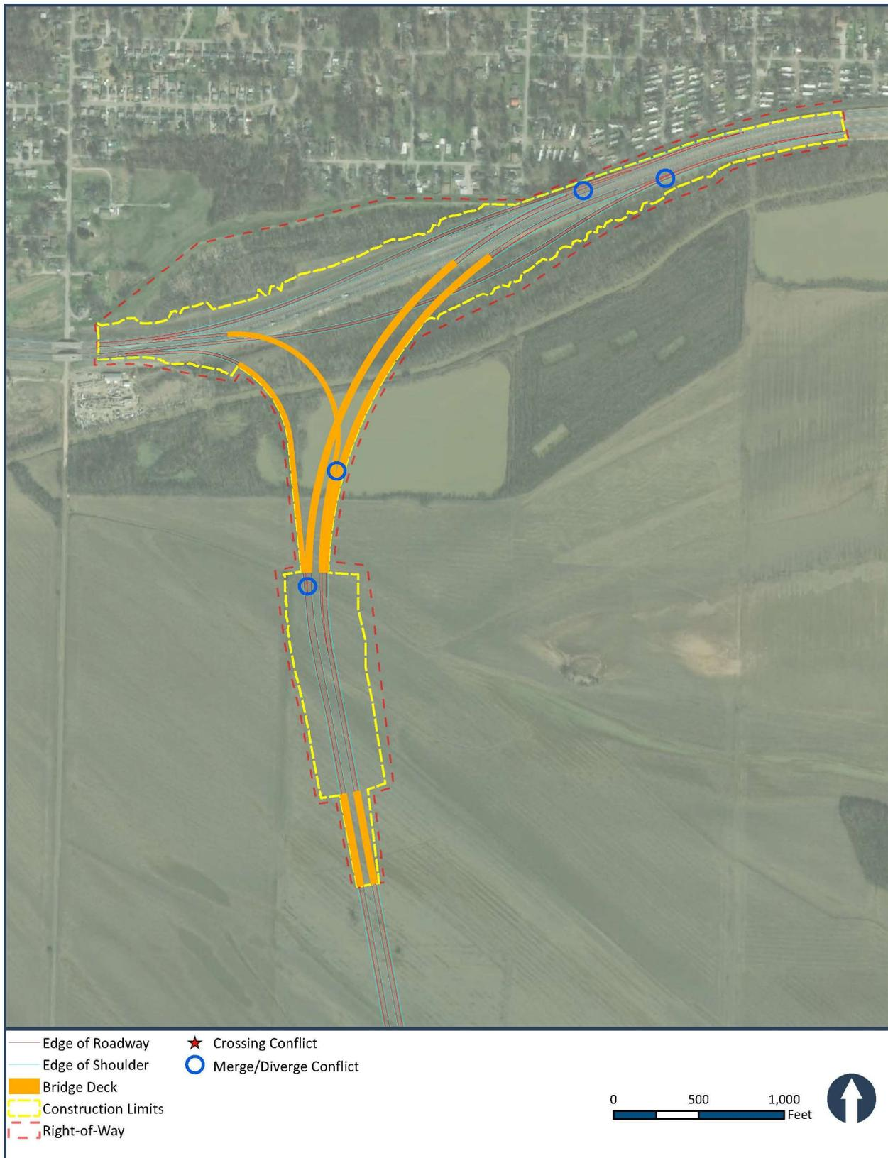
**Figure 2-3. VMP Concept C: System Interchange with Left-Hand Exit**
