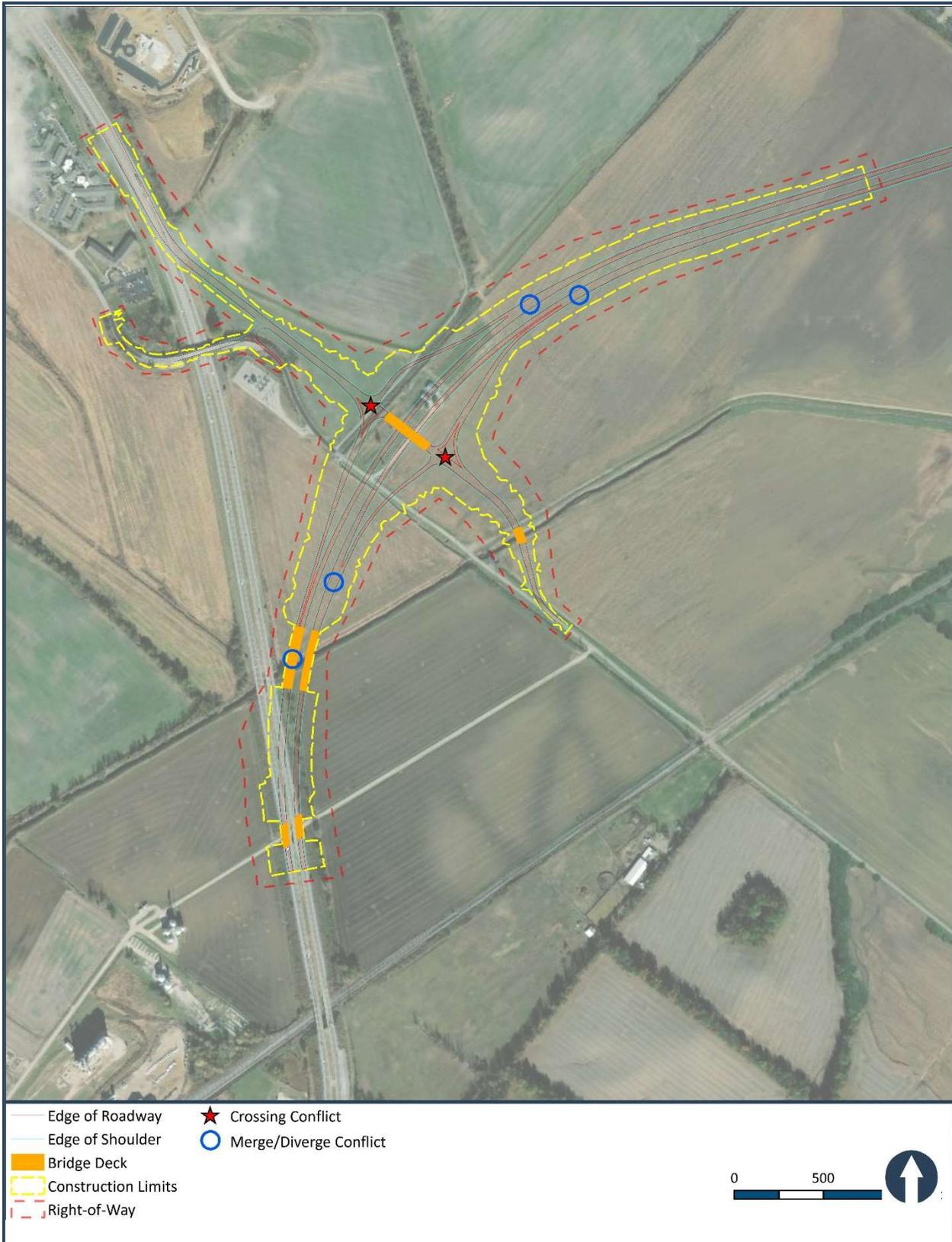
**Figure 4-4. US 41 Concept D: Diamond Interchange 2 (Service Interchange)**
