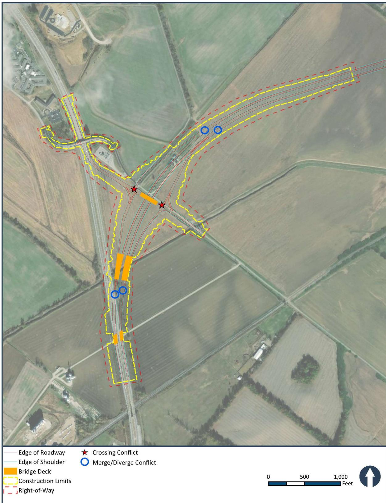
**Figure 4-3. US 41 Concept C: Diamond Interchange 1 (Service Interchange)**
